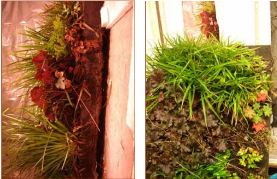
Figure 5.60 Living wall based on mineral wool panels as placed inside the climate chamber. The air cavity between panels and façade was 5 cm. Plant species used: Ferns, Geraniums and Carex.
