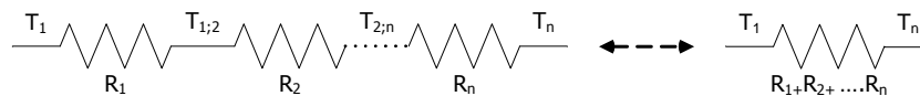
Figure 5.2 Thermal resistances of separate layers of a construction can be schematized as a (electrical) series system.
