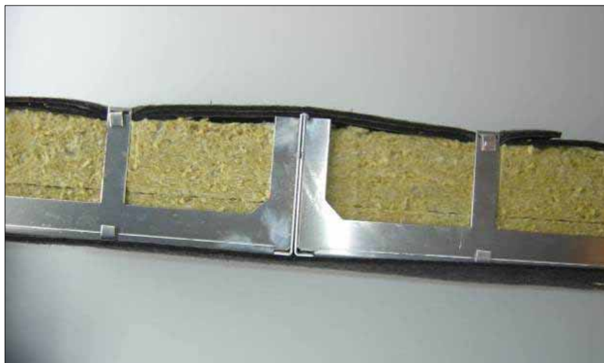
Figure 5.61 Cross section of the living wall panel filled with mineral wool as substrate.
