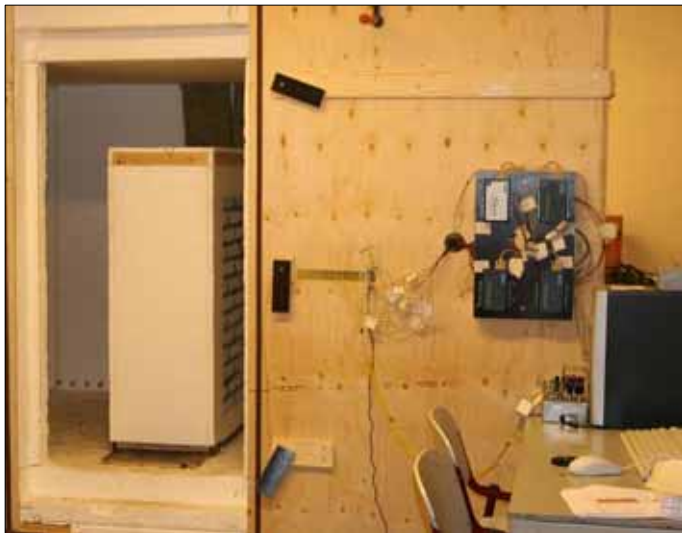
Figure 5.23 The bare wall as placed inside the designed apparatus, dividing the box into two chambers, the outside chamber (right handed) and the inside chamber (left handed). On this way two different climates can be achieved and simulated.
