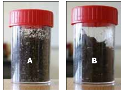
Figure 4.6.4 Soil samples from porous concrete layer, photo A is initial soil, photo B soil after three months of installation.
