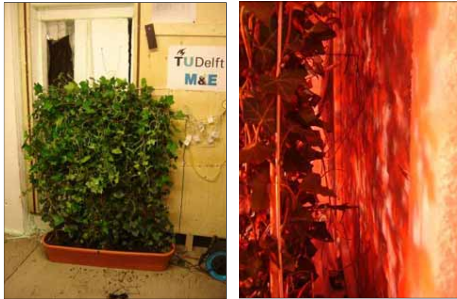
Figure 5.38 Roughly 1 m 2 of Hedera helix placed in a container filled with soil to ensure the plants vitality during the measurements inside the box. The climber attached to a trellis was mounted 10 cm from the façade to guarantee an air cavity and simulate indirect façade greenery.
