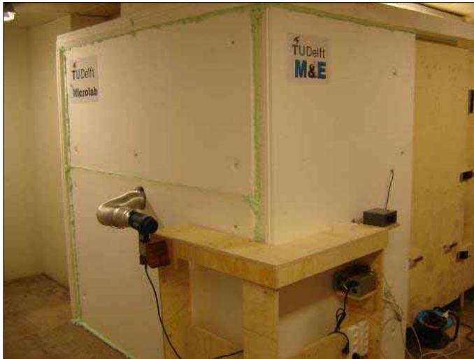
Figure 5.25 The climate chamber where the heating or cooling energy is generated, is protected against the influence of the environment with an extra guard (cavity with the same temperature as inside the climate chamber to avoid energy losses). On this way an adiabatic environment is created.
