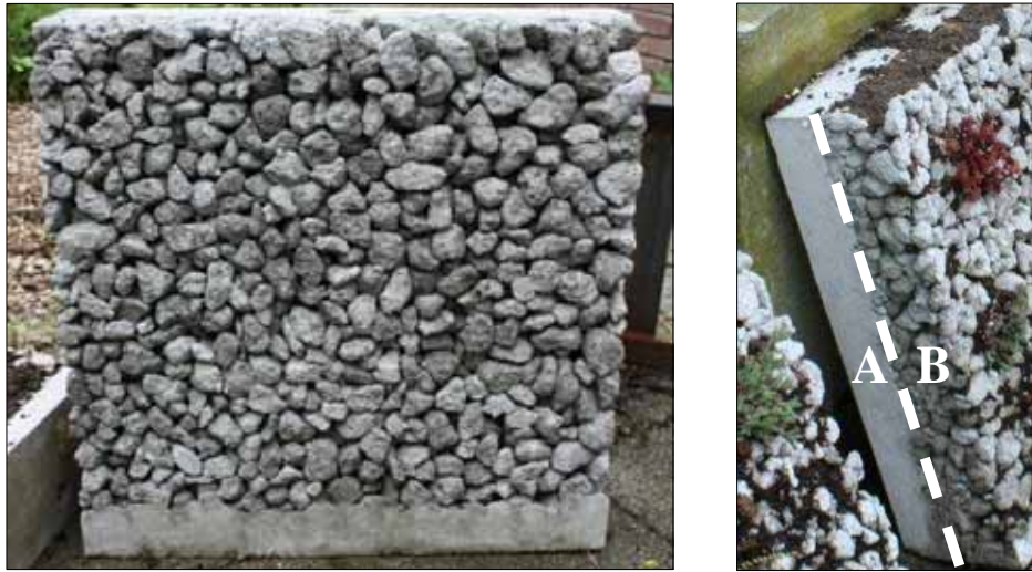
Figure 4.6.1 Green concrete prototype block created for plant growth.
