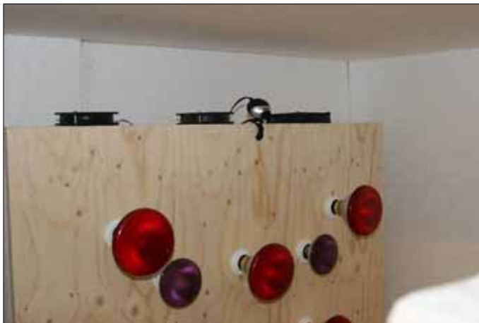
Figure 5.26 Panel with infrared bulbs (red) to simulate radiation and growing bulbs (purple) to maintain an "optimal" condition for the plants (when the box is closed no light is available for photosynthesis, since a greening system is roughly two weeks inside the box artificial light is necessary to keep the plants alive during the measuring period).
