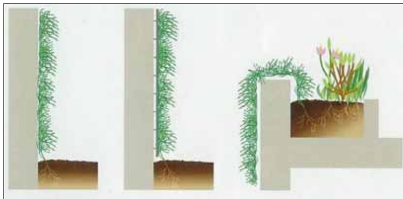
Figure 4.2.1 Different types of façade greening (according to Hermy et al., 2005).
