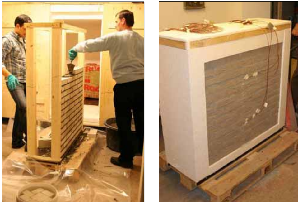
Figure 5.20 Left photograph; building of the bare wall as used for the measurements. Right photograph; the bare wall as a package of 1 m 2 ready for placement inside the designed apparatus.
