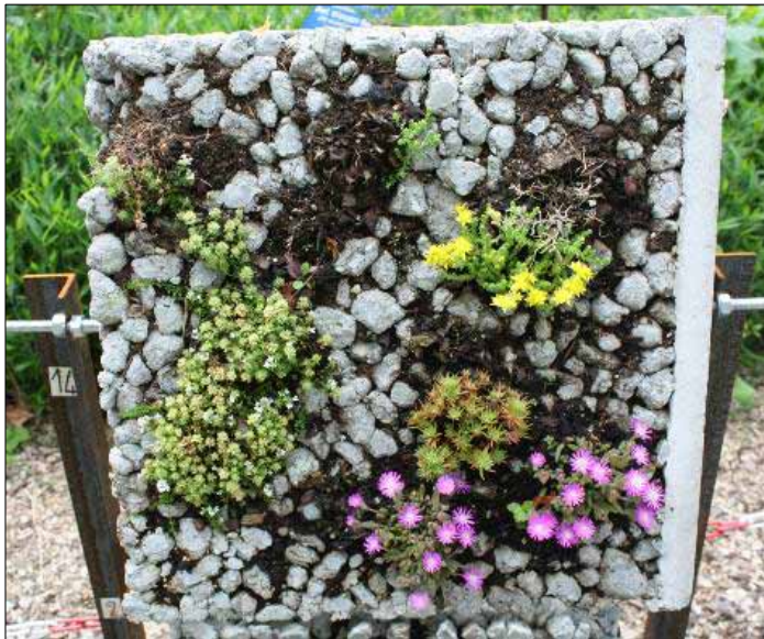
Figure 3.4b Porous concrete intended as growing medium for plants and to stimulate the colonization of different plant species.
