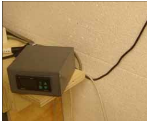
Figure A.9: Pt-100, temperature measurement supply.
