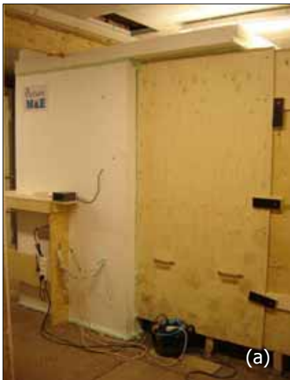
Figure 4.5: (a) outside EPS-insulation layer with an air cavity around the hotbox; (b) measuring computer outside the hotbox.
