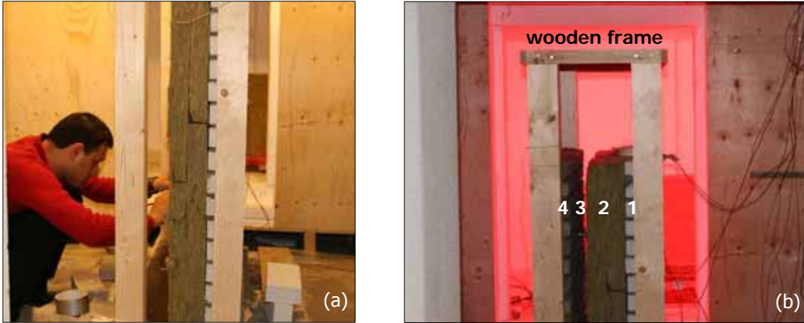
Figure 4.6: (a) the test specimen during the building process; (b) the side view of test specimen: 1- inner leaf; 2- insulation; 3- air cavity and 4- masonry.
