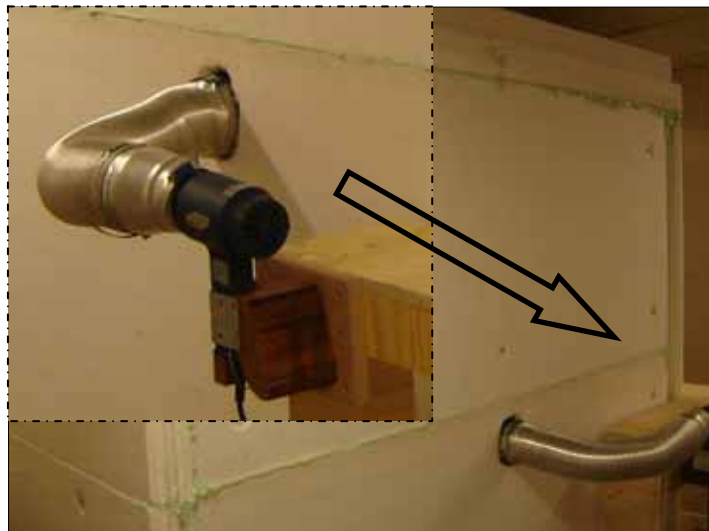
Figure A.7: Hot-air gun connection with an aluminium pipe, outside the hotbox.
