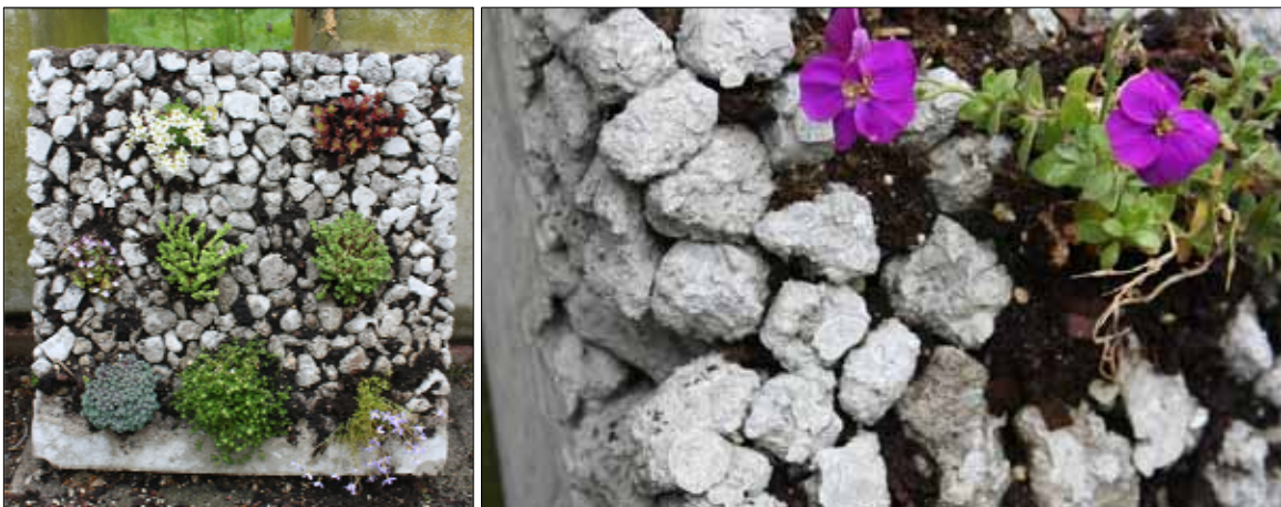
Figure 2.16: concrete panels (Growcrete) with plants (source: Ottel , 2010).
