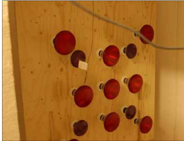
Figure A.6: IR lights (red and big size), plant reflector lamps (rose and small size) on the same panel.
