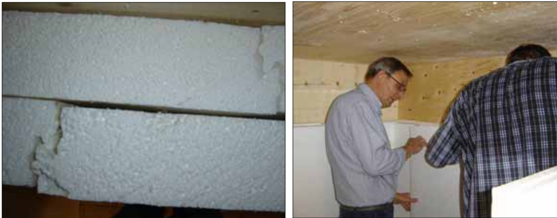
Figure 4.2: left, two layers of EPS glued to each other; right, technicians during the building of hotbox.
