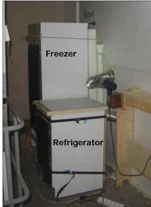
Figure A.8: A refrigerator (cooling unit) used for outside air cavity (insulation cover around the hotbox) and a high performance 'SIEMENS' freezer for inside the hotbox.
