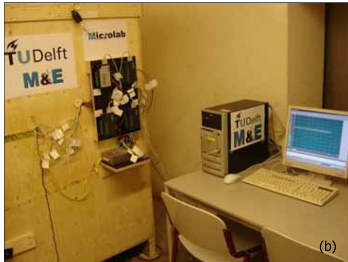
Figure 4.5: (a) outside EPS-insulation layer with an air cavity around the hotbox; (b) measuring computer outside the hotbox.
