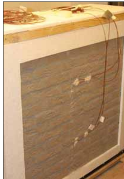
Figure A.2: thermocouples (brown wires) used through the test specimen.
